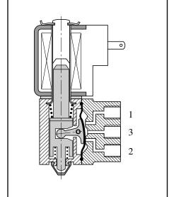
The connection ports are shown in vertical position in order to make the operation easier to understand.
